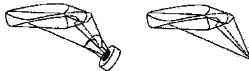
Fig. 8A Diagram of a wave guide with real and theoretical parabolic reflecting surfaces
