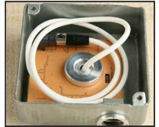
Fig F. Set the initial height of the M3 and spool the excess cable inside the junction box.
