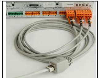
Fig L. Connect RJ45 cables into the breakout cable and connect to DSP Controller.
